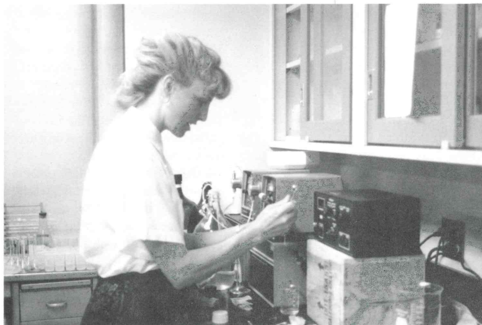
New Mexico Tech graduate student Michelle Cash uses high-performance liquid chromatography to analyze air quality samples (Air Quality Studies in Albuquerque, Report No. 275).
